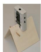
For electric fields measurements, use the ungrounded (potential-free) instrument, i.e. NOT connected with the grounding wire, NOT held in the hand but placed on a non-conductive holder (preferable use dry wood or cardboard) or non-conductive handle of at least 1.5m (5ft). View the instruments reading from a distance of at least 1.5m (5ft). Place the instrument on the holder and rotate/move the holder accordingly.
